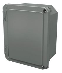
Stahlin Diamond Shield series enclosure, NEMA 1/3/3S/4X/12/13, 8 x 6 x 4in (HxWxD), wall mount, fiberglass reinforced polyester, gray, crowned hinged screw cover.
