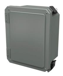
Stahlin Diamond Shield series enclosure, NEMA 1/3/3S/4X/12/13,  $8 \times 6 \times 4$  in (HxWxD), wall mount, fiberglass reinforced polyester, gray, crowned single-door, (2) quick-release latches, padlock hasp and staple.
