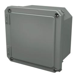
Stahlin Diamond Shield series enclosure, NEMA 1/3/3S/4X/12/13, 6 x 6 x 4in (HxWxD), wall mount, fiberglass reinforced polyester, gray, crowned screw cover.
