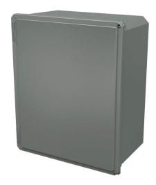
Stahlin Diamond Shield series enclosure, NEMA 1/3/3S/4X/12/13, 20 x 16 x 10in (HxWxD), wall mount, fiberglass reinforced polyester, gray, crowned hinged screw cover.
