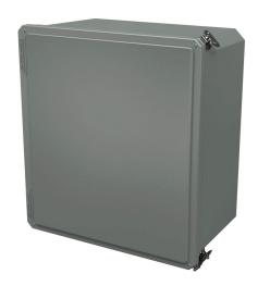
Stahlin Diamond Shield series enclosure, NEMA 1/3/3S/4X/12/13,  $18 \times 16 \times 10$  in (HxWxD), wall mount, fiberglass reinforced polyester, gray, crowned single-door, (2) twist-lock latches, padlock hasp and staple.
