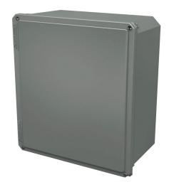
Stahlin Diamond Shield series enclosure, NEMA 1/3/3S/4X/12/13, 16 x 14 x 8in (HxWxD), wall mount, fiberglass reinforced polyester, gray, crowned screw cover.
