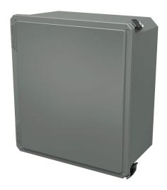
Stahlin Diamond Shield series enclosure, NEMA 1/3/3S/4X/12/13,  $16 \times 14 \times 8$  in (HxWxD), wall mount, fiberglass reinforced polyester, gray, crowned single-door, (2) quick-release latches, padlock hasp and staple.
