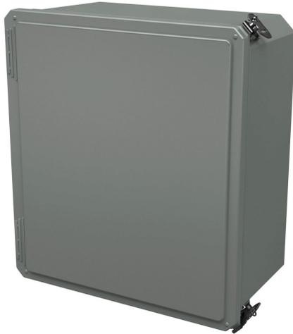
Stahlin Diamond Shield series enclosure, NEMA 1/3/3S/4X/12/13, 16 x 14 x 8in (HxWxD), wall mount, fiberglass reinforced polyester, gray, crowned single-door, (2) twist-lock latches, padlock hasp and staple.
