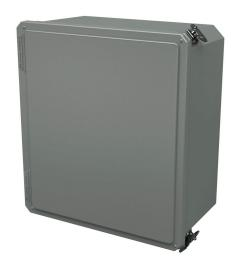
Stahlin Diamond Shield series enclosure, NEMA 1/3/3S/4X/12/13,  $16 \times 14 \times 8$  in (HxWxD), wall mount, fiberglass reinforced polyester, gray, crowned single-door, (2) twist-lock latches, padlock hasp and staple.
