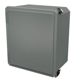
Stahlin Diamond Shield series enclosure, NEMA 1/3/3S/4X/12/13,  $14 \times 12 \times 8$  in (HxWxD), wall mount, fiberglass reinforced polyester, gray, crowned single-door, (2) quick-release latches, padlock hasp and staple.
