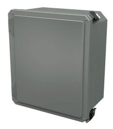
Stahlin Diamond Shield series enclosure, NEMA 1/3/3S/4X/12/13,  $12 \times 10 \times 6$  in (HxWxD), wall mount, fiberglass reinforced polyester, gray, crowned single-door, (2) quick-release latches, padlock hasp and staple.
