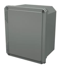
Stahlin Diamond Shield series enclosure, NEMA 1/3/3S/4X/12/13, 10 x 8 x 6in (HxWxD), wall mount, fiberglass reinforced polyester, gray, crowned screw cover.
