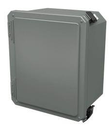
Stahlin Diamond Shield series enclosure, NEMA 1/3/3S/4X/12/13,  $10 \times 8 \times 6$  in (HxWxD), wall mount, fiberglass reinforced polyester, gray, crowned single-door, (2) quick-release latches, padlock hasp and staple.
