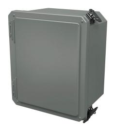
Stahlin Diamond Shield series enclosure, NEMA 1/3/3S/4X/12/13,  $10 \times 8 \times 6$  in (HxWxD), wall mount, fiberglass reinforced polyester, gray, crowned single-door, (2) twist-lock latches, padlock hasp and staple.
