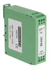
Roxburgh EMI input filter, 120/240 VAC, 1-phase, 8A, 35mm DIN rail mount, EMI/RFI filtering, 1-stage, general purpose, standard performance, screw terminals.
