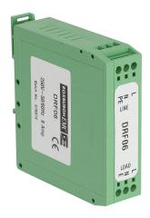
Roxburgh EMI input filter, 120/240 VAC, 1-phase, 6A, 35mm DIN rail mount, EMI/RFI filtering, 1-stage, general purpose, standard performance, screw terminals.
