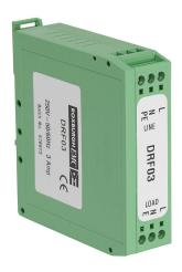
Roxburgh EMI input filter, 120/240 VAC, 1-phase, 3A, 35mm DIN rail mount, EMI/RFI filtering, 1-stage, general purpose, standard performance, screw terminals.
