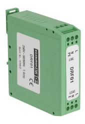
Roxburgh EMI input filter, 120/240 VAC, 1-phase, 1A, 35mm DIN rail mount, EMI/RFI filtering, 1-stage, general purpose, standard performance, screw terminals.
