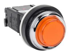
Fuji Electric LED indicating light, permanent light function, 30mm, orange, 41mm, extended round, plastic base, metal bezel, 115-127 VAC, transformer.
