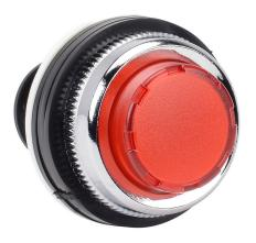
Fuji Electric LED indicating light, permanent light function, 30mm, red, 41mm, extended round, plastic base, metal bezel, 24 VAC/VDC, full voltage.
