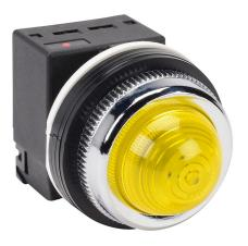
Fuji Electric LED indicating light, permanent light function, 30mm, yellow, 41mm, dome, plastic base, metal bezel, 115-127 VAC, transformer.
