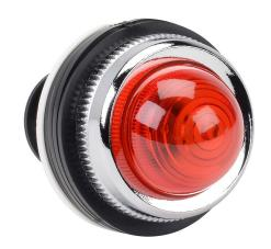
Fuji Electric LED indicating light, permanent light function, 30mm, red, 41mm, dome, plastic base, metal bezel, 24 VAC/VDC, full voltage.
