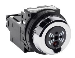
Fuji Electric audible alarm buzzer, 90 dB at 0.1m, 70 dB at 1m, 2.4 kHz to 3.3 kHz tone frequency, continuous/intermittent tone(s), 100 to 110 VAC, permanent LED indicator(s), red, 30mm, panel mount, plastic housing, silver, IP00.
