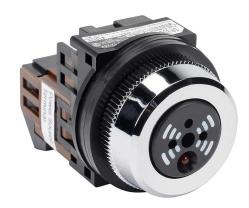
Fuji Electric audible alarm buzzer, 90 dB at 0.1m, 70 dB at 1m, 2.4 kHz to 3.3 kHz tone frequency, continuous/intermittent tone(s), 12-24 VAC/VDC, permanent LED indicator(s), red, 30mm, panel mount, plastic housing, silver, IP00.
