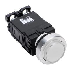
Fuji Electric LED indicating light, permanent light function, IP65, 22mm, white, 30mm, round, plastic base, metal bezel, 115-127 VAC, transformer.
