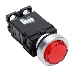
Fuji Electric LED indicating light, permanent light function, IP65, 22mm, red, 30mm, round, plastic base, metal bezel, 115-127 VAC, transformer.
