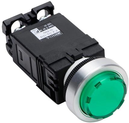
Fuji Electric LED indicating light, permanent light function, IP65, 22mm, green, 24mm, round, plastic base, metal bezel, 115-127 VAC, transformer.
