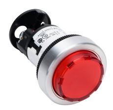
Fuji Electric LED indicating light, permanent light function, IP65, 22mm, red, 30mm, round, plastic base, metal bezel, 24 VAC/VDC, full voltage.
