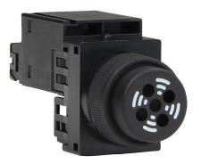
Fuji Electric audible alarm buzzer, 80 dB at 0.1m, 60 dB at 1m, 2.4 kHz to 3.3 kHz tone frequency, continuous/intermittent tone(s), 100-110 VAC, 22mm, panel mount, plastic housing, black, IP54.
