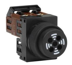
Fuji Electric audible alarm buzzer, 80 dB at 0.1m, 60 dB at 1m, 2.4 kHz to 3.3 kHz tone frequency, continuous/intermittent tone(s), 12 to 24 VAC/VDC, 22mm, panel mount, plastic housing, black, IP54.
