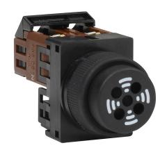
Fuji Electric audible alarm buzzer, 80 dB at 0.1m, 60 dB at 1m, 2.4 kHz to 3.3 kHz tone frequency, continuous/intermittent tone(s), 12-24 VAC/VDC, 22mm, panel mount, plastic housing, black, IP54.
