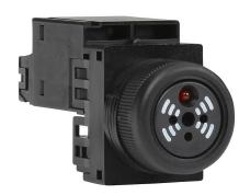
Fuji Electric audible alarm buzzer, 90 dB at 0.1m, 70 dB at 1m, 2.4 kHz to 3.3 kHz tone frequency, continuous/intermittent tone(s), 100-110 VAC, permanent LED indicator(s), red, 22mm, panel mount, plastic housing, black, IP00.
