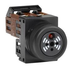
Fuji Electric audible alarm buzzer, 90 dB at 0.1m, 70 dB at 1m, 2.4 kHz to 3.3 kHz tone frequency, continuous/intermittent tone(s), 12-24 VAC/VDC, permanent LED indicator(s), red, 22mm, panel mount, plastic housing, black, IP00.
