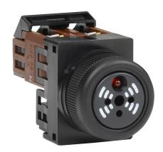
Fuji Electric audible alarm buzzer, 90 dB at 0.1m, 70 dB at 1m, 2.4 kHz to 3.3 kHz tone frequency, continuous/intermittent tone(s), 12 to 24 VAC/VDC, permanent LED indicator(s), red, 22mm, panel mount, plastic housing, black, IP00.
