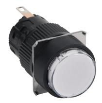
Fuji Electric LED indicating light, permanent light function, IP65, 16mm, white, 18mm, round, plastic base, plastic bezel, 24 VAC/VDC, full voltage.
