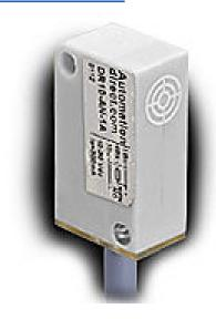
Micro Detectors inductive proximity sensor, rectangular,  $10.3 \times 28 \times 16$ mm body, polyphthalamide housing, NPN, N.O. output, 6mm sensing distance, non-flush, 3 kHz switching frequency, IP67, pigtail.
