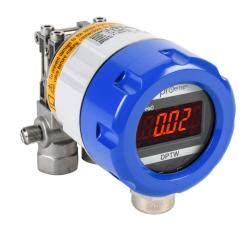
ProSense differential pressure transmitter, 0 to 8in of water column range, 4-20 mA analog output, 1/4in female NPT process connection, 12-32 VDC operating voltage, screw terminals, panel or wall mount.
