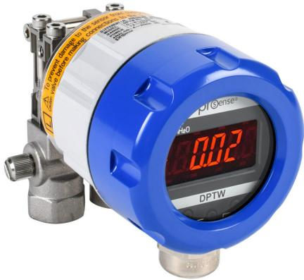
ProSense differential pressure transmitter, 0 to 80in of water column range, 4-20 mA analog output, 1/4in female NPT process connection, 12-32 VDC operating voltage, screw terminals, panel or wall mount.
