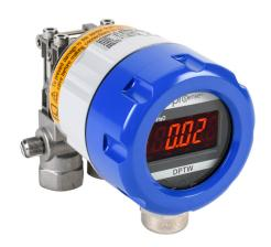
ProSense differential pressure transmitter, 0 to 4in of water column range, 4-20 mA analog output, 1/4in female NPT process connection, 12-32 VDC operating voltage, screw terminals, panel or wall mount.
