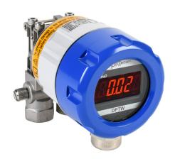
ProSense differential pressure transmitter, 0 to 20in of water column range, 4-20 mA analog output, 1/4in female NPT process connection, 12-32 VDC operating voltage, screw terminals, panel or wall mount.
