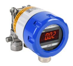
ProSense differential pressure transmitter, 0 to 200in of water column range, 4-20 mA analog output, 1/4in female NPT process connection, 12-32 VDC operating voltage, screw terminals, panel or wall mount.
