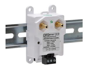
ProSense air differential pressure transmitter, -0.5 to +0.5in of water column range, 4-20 mA analog output, 1/4in brass barbed process connection, 12 to 36 VDC operating voltage, screw terminals, 35mm DIN rail or panel mount.
