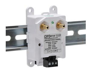
ProSense air differential pressure transmitter, 0 to 0.25in of water column range, 4-20 mA analog output, 1/4in brass barbed process connection, 12 to 36 VDC operating voltage, screw terminals, 35mm DIN rail or panel mount.
