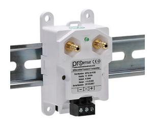
ProSense air differential pressure transmitter, -0.25 to +0.25in of water column range, 4-20 mA analog output, 1/4in brass barbed process connection, 12 to 36 VDC operating voltage, screw terminals, 35mm DIN rail or panel mount.
