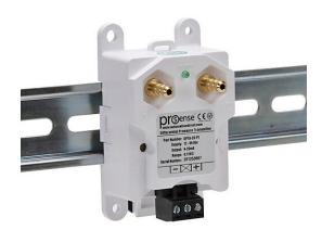
ProSense air differential pressure transmitter, 0 to 0.1in of water column range, 4-20 mA analog output, 1/4in brass barbed process connection, 12 to 36 VDC operating voltage, screw terminals, 35mm DIN rail or panel mount.
