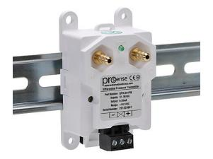
ProSense air differential pressure transmitter, -0.1 to +0.1in of water column range, 4-20 mA analog output, 1/4in brass barbed process connection, 12 to 36 VDC operating voltage, screw terminals, 35mm DIN rail or panel mount.
