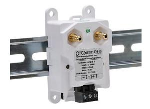
ProSense air differential pressure transmitter, 0 to 25.0in of water column range, 4-20 mA analog output, 1/4in brass barbed process connection, 12 to 36 VDC operating voltage, screw terminals, 35mm DIN rail or panel mount.
