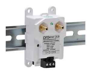
ProSense air differential pressure transmitter, 0 to 15.0in of water column range, 4-20 mA analog output, 1/4in brass barbed process connection, 12 to 36 VDC operating voltage, screw terminals, 35mm DIN rail or panel mount.
