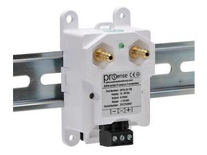
ProSense air differential pressure transmitter, -15.0 to +15.0 in of water column range, 4-20 mA analog output, 1/4in brass barbed process connection, 12 to 36 VDC operating voltage, screw terminals, 35mm DIN rail or panel mount.
