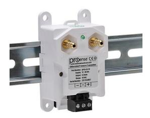
ProSense air differential pressure transmitter, 0 to 10.0in of water column range, 4-20 mA analog output, 1/4in brass barbed process connection, 12 to 36 VDC operating voltage, screw terminals, 35mm DIN rail or panel mount.
