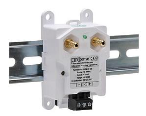
ProSense air differential pressure transmitter, -10.0 to +10.0in of water column range, 4-20 mA analog output, 1/4in brass barbed process connection, 12 to 36 VDC operating voltage, screw terminals, 35mm DIN rail or panel mount.
