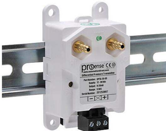
ProSense air differential pressure transmitter, 0 to 5.0in of water column range, 4-20 mA analog output, 1/4in brass barbed process connection, 12 to 36 VDC operating voltage, screw terminals, 35mm DIN rail or panel mount.
