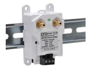
ProSense air differential pressure transmitter, -5.0 to +5.0in of water column range, 4-20 mA analog output, 1/4in brass barbed process connection, 12 to 36 VDC operating voltage, screw terminals, 35mm DIN rail or panel mount.
